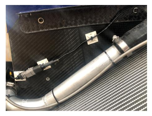
7. Ensure all wires are out of harms way and especially the camera loom wire around the hole in the engine cover.
