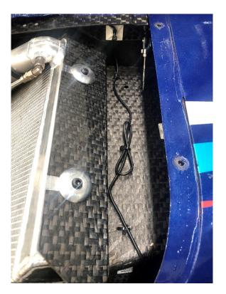
6. Route cable as shown, adding cable tie mounts. And connect back into the car loom.
