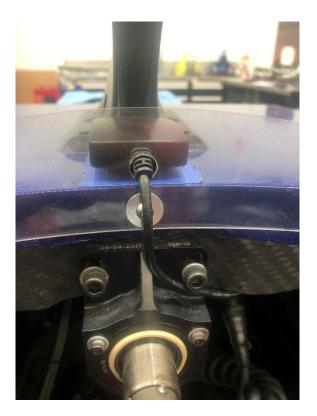
4. Route cable along the existing loom through the hole in the chassis on the RHS underneath the seat
