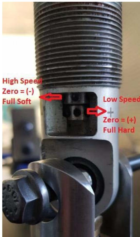
When setting these adjusters, please use the JRi pin tool (GRM-CI0002-00) to not overtighten & jam the adjuster. These are designed to snap if forced too hard. The tool can be ground flat & re-used if the dowel pin remains with sufficient length. New pin tools are available to purchase.
