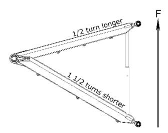
As a result of this shortening of Mechanical Trial, Camber stays unchanged, and Caster decreases by 0.8°.
