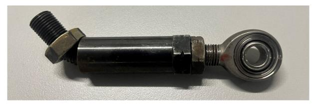
The current failure mode with the significant bending of the adjusters is not ideal as a large variation in push rod and steering arm length occurs as a result.
