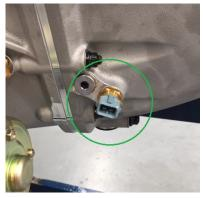
The oil level is to the bottom of this fill hole and the oil capacity is approximately 0.5L.
