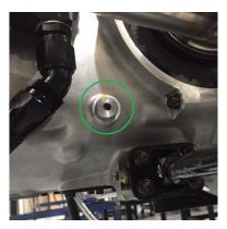
When filled from dry, and after the first transmission run up, the oil level will need to be topped up to the correct fill level. The capacity is approximately 3.5L.
