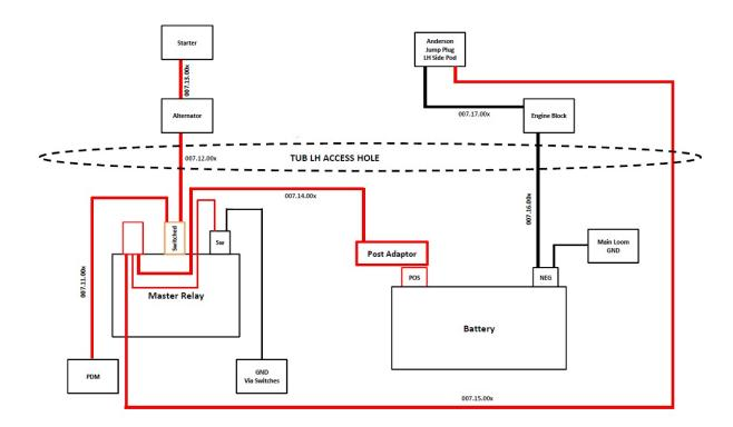
An Anderson Jump plug is located in the left-hand side pod for connection of an auxiliary battery. It is recommended an auxiliary battery is connected at all times the car is turned on without the engine running.
