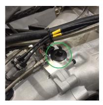
The oil level is set to the bottom of the RH level plug.
