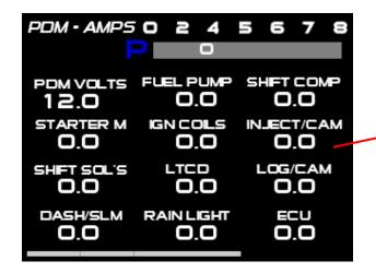
Displays the current being output by the PDM.
