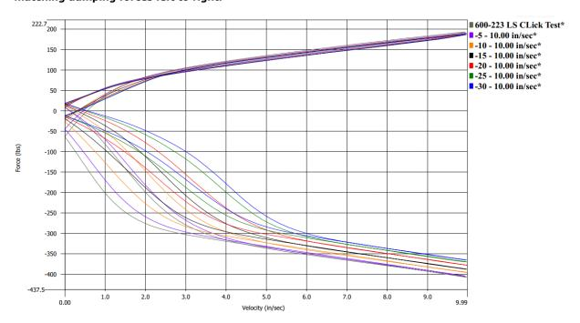
Occasionally due to manufacturing tolerances, not all shocks supplied will have equal shock settings for the same forces. Please confirm with GRM if your set has unequal settings.
