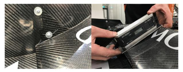
Lower Rear wing adjustment and measurement
