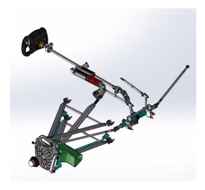
The rear suspension of the S5000 is unequal length double wishbone with an upper toe link to control toe angle. As with the front suspension, the rear coil over dampers and adjustable anti-roll bar are actuated by a pushrod and rocker mechanism.
