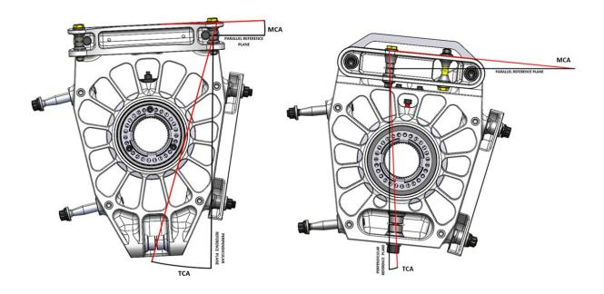
The Castor Angle influences the Castor Offset/Mechanical Trail and therefore the force to turn the wheel. Castor Offset is along the ground plane while the Mechanical Trail is perpendicular to the steering axis.
