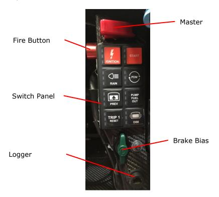
MASTER SWITCH: Toggle Switch, turns the Car on (switch to the right) and off
