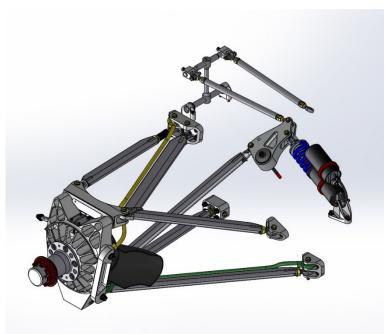
There is only a single spring and damper per wheel, there is no third element or interconnection between front and rear suspensions. In addition to the coil over spring, each damper has a bump rubber and packer system.
