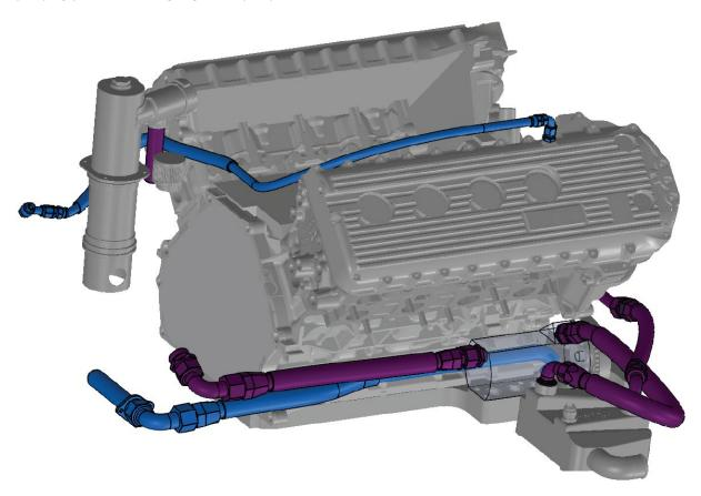
Below 50°C engine oil temperature the engine management system limits the maximum engine speed to 2500rpm. The maximum oil temperature must not exceed 120°C.
