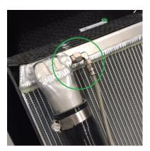
Once air has finished escaping from the top of the RH radiator, reconnect the fitting and continue filling the system until the header tank/swirl pot is approximately  $\frac{3}{4}$  full when engine is cold.
